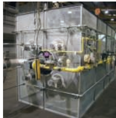
FIGURE 5. Direct-fired oxidizers may be the preferred emission-control solution when there is a very high VOC or hydrocarbon load, as well as fluctuating operating conditions
