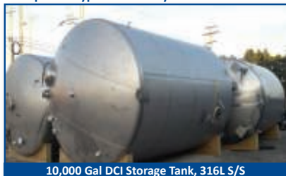
10,000 Gal DCI Storage Tank, 316L S/S
